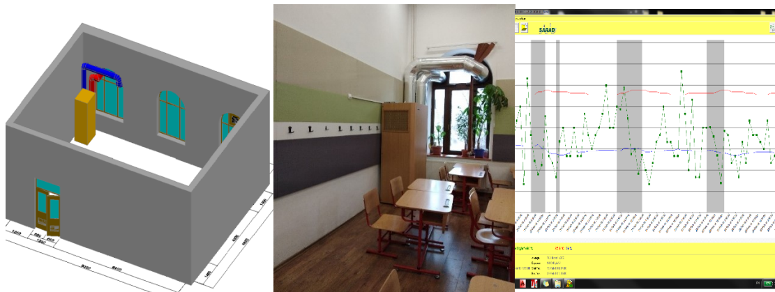
Figure 1 A 3D Model of the classroom B.Heat recovery ventilation unit photo C.Radon measurements
